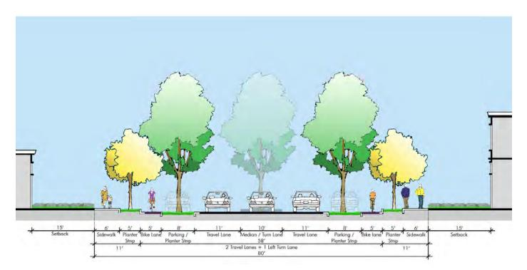
Figure 3.6: Franklin Boulevard, Sacramento, CA – Proposed Prototypical Section (Looking North)
