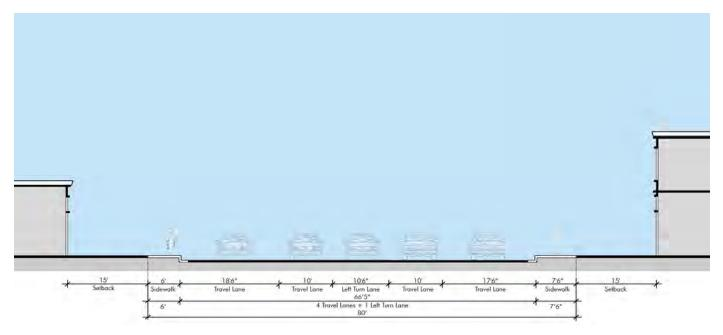
**Figure 3.4: North Franklin Boulevard, Sacramento, CA – Existing Prototypical Section (Looking North)** Drawings and simulations courtesy of MIG Consulting Services
