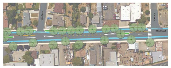
Figure 3.9: 24th Street Streetscape Road Diet Conceptual Layout Reduces Four Lanes of Traffic to Two Lanes
